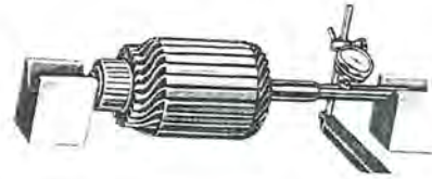
Fig. 18-Checking Armature for Bent Shaft
