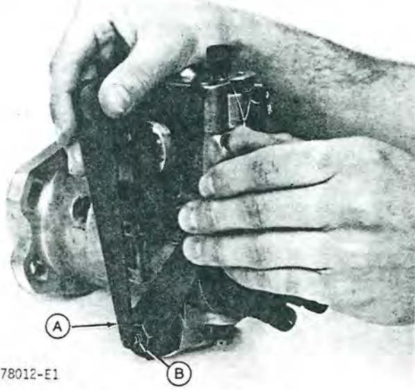
Fig. 14-Adjusting Speed Advance (6466D Engine) (Pump removed for illustrative purposes)
